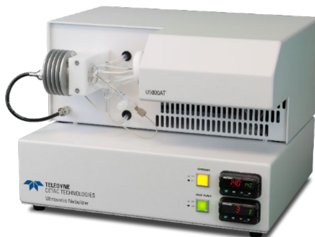
Figure 1. Teledyne CETAC Technologies U5000AT+ Ultrasonic Nebulizer (USN)
