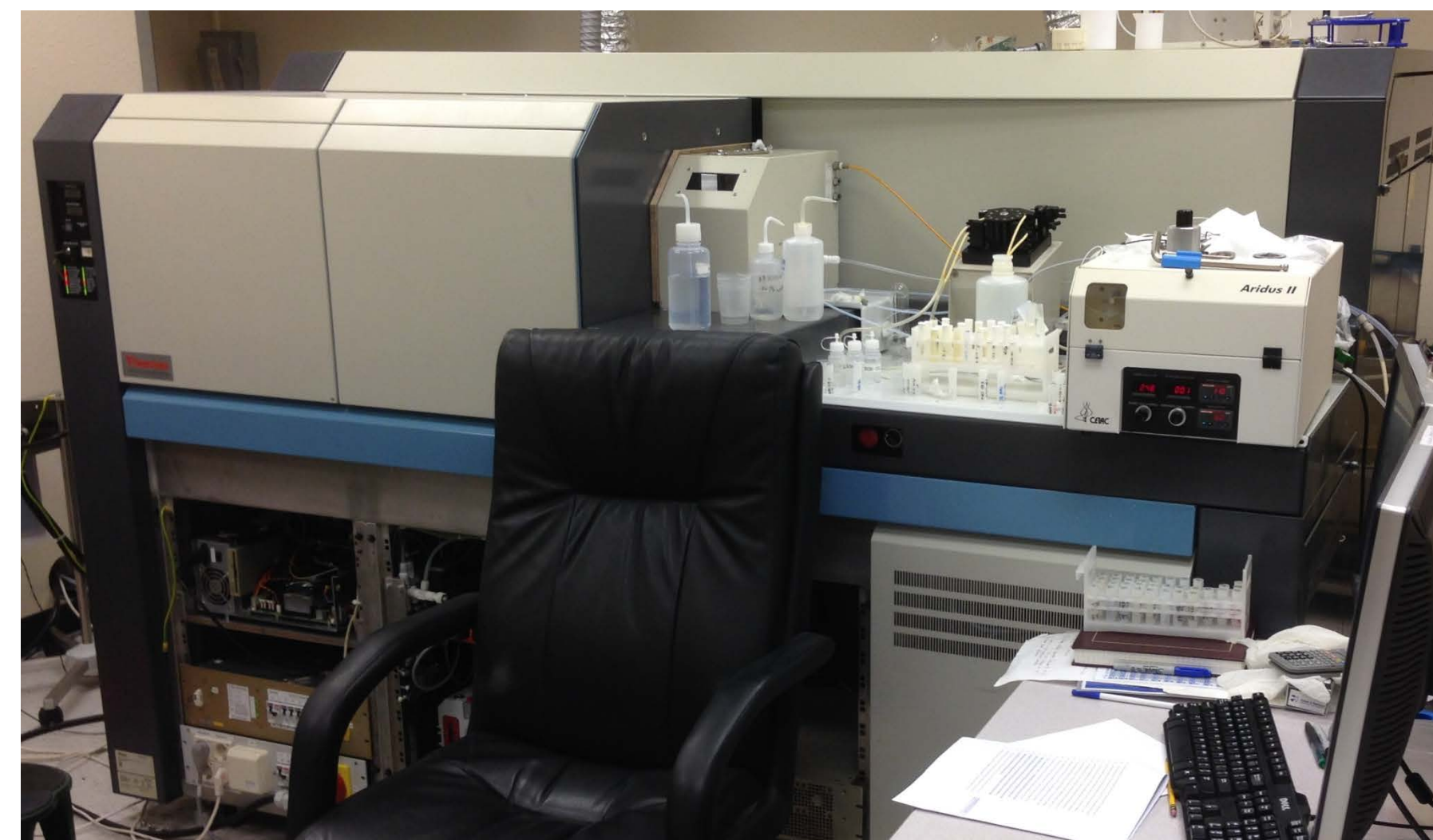
Figure 4. Thermo Neptune MC-ICP-MS & Teledyne CETAC AridusII Desolvating Nebulizer System
