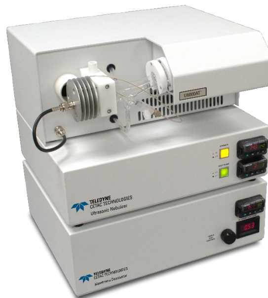
Figure 1. Teledyne CETAC U6000AT+ USN/Membrane Desolvator
