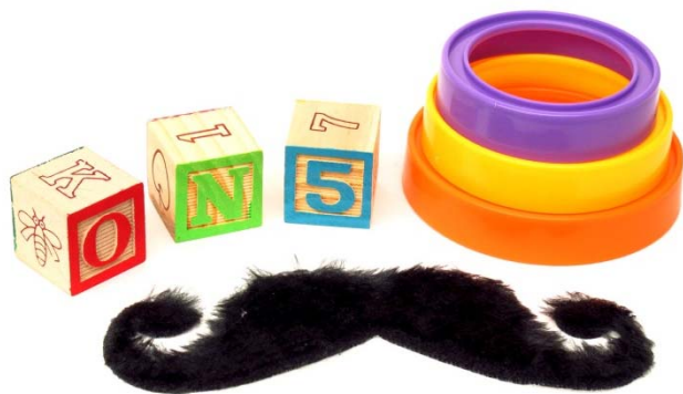
Figure 1. Assorted toy samples include painted wooden blocks, plastic stacking rings, and a fake moustache. All samples are EN-71 Part 3 Category III sample types.
