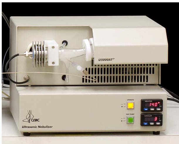
Figure 2b. Teledyne CETAC U5000AT + USN in operation
