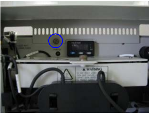
23. Tighten thumbscrew to secure cover.
