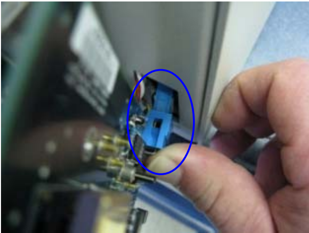
14. Line up new board connector with cable connector.
