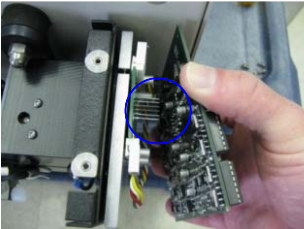
11. Acq. Board slides off the six connecting pins.
