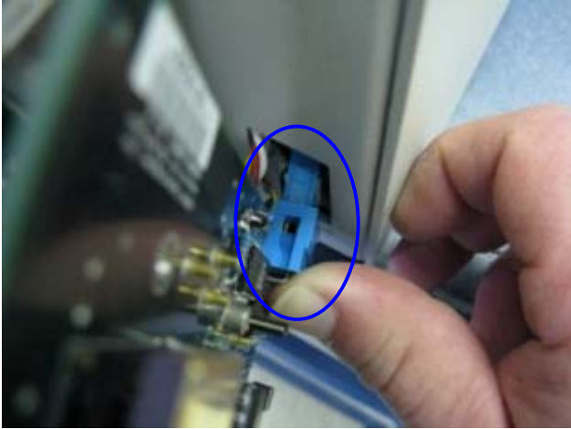
21. Line up Acq. board connector with cable connector.
