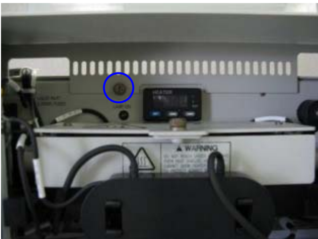
30. Tighten thumbscrew to secure cover.
