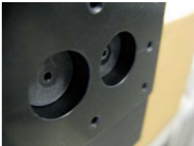
18. Remove the burnt filters from the camera block.
