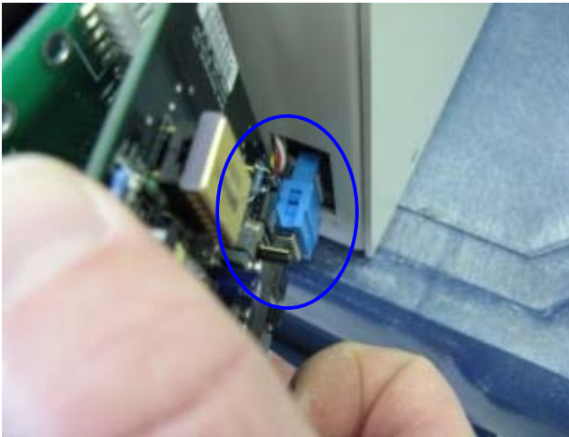
13. Gently rock and pull forward to remove from data connection.
