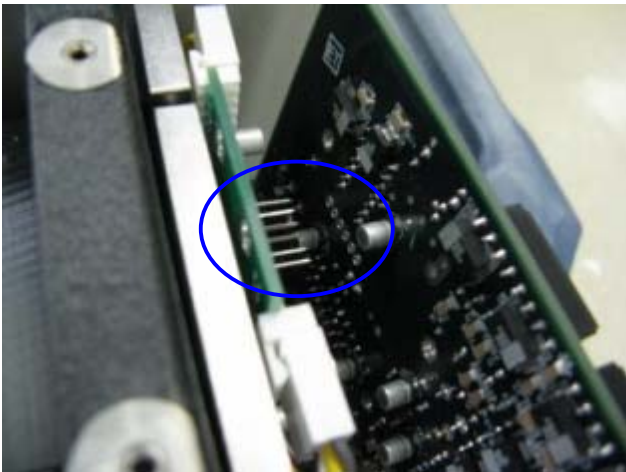
25. Carefully align the six pins and their contact points.
