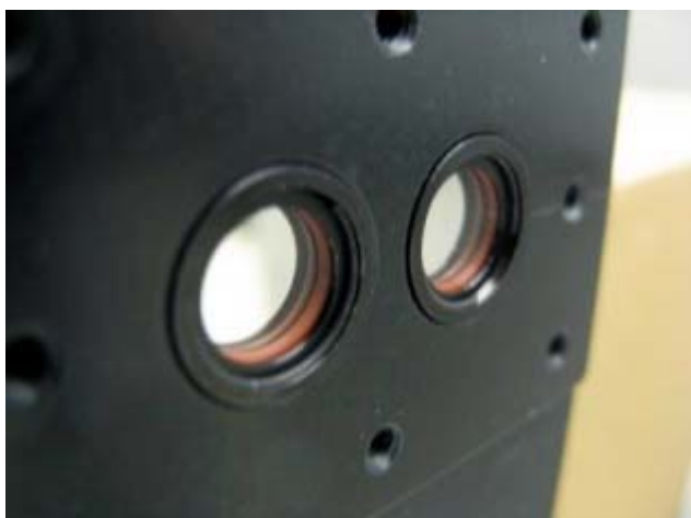
19. Ensure filters are clean(both sides), no particulate or fingerprints. Insert the new filters as shown.
