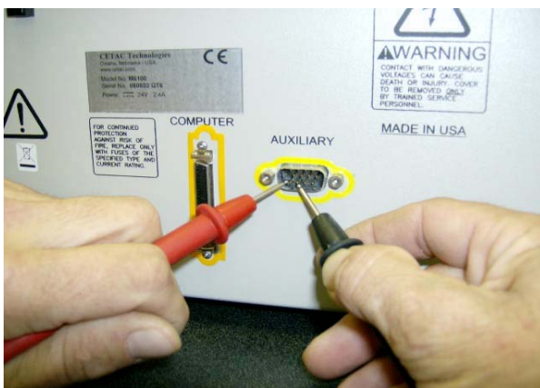
Using a voltmeter on auxiliary pins 6 & 7
