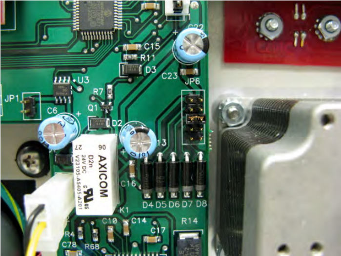
Figure 19. Pump Speed Jumpers at JP6.
