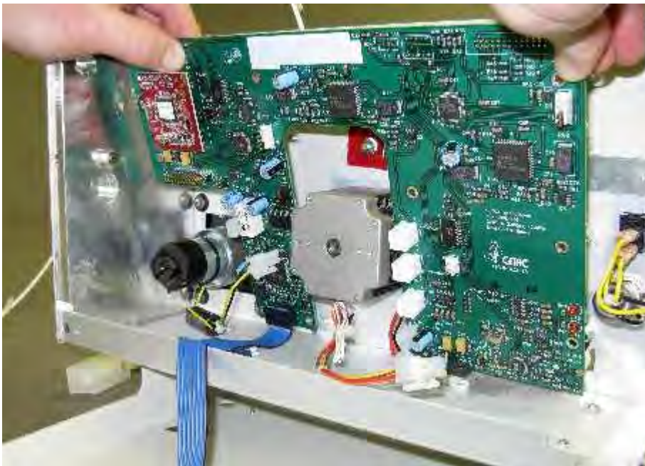
Figure 18. Removing the main board. Rabbit processor is the small board in the top left corner.
