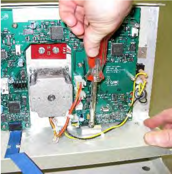
Figure 15. Removing the voltage regulator heat sink.
