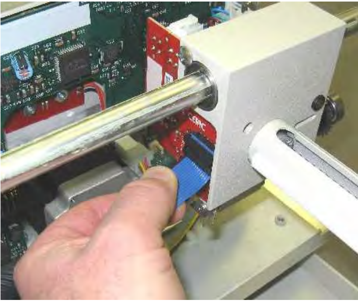
Figure 11. Removal of blue ribbon cable from carriage.
