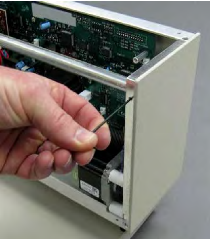
Figure 12. Loosening of guide shaft set screw.
