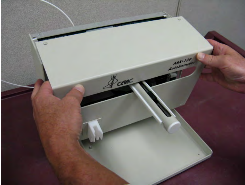
Figure 8. View of ASX-130 Autosampler with the front cover being removed.
