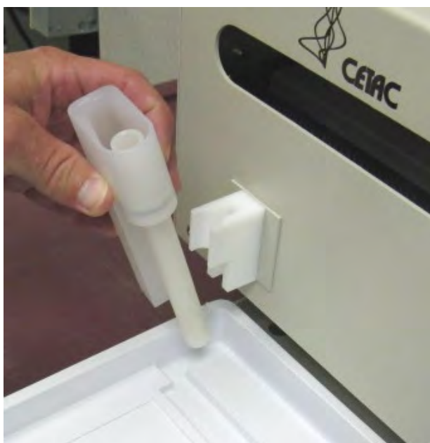
Figure 4. View of rinse station.
