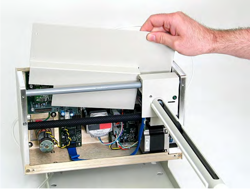
Figure 10. Removal of inner shield.
