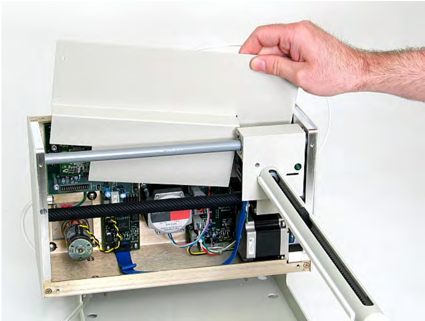
Figure 10. Removal of inner shield.
