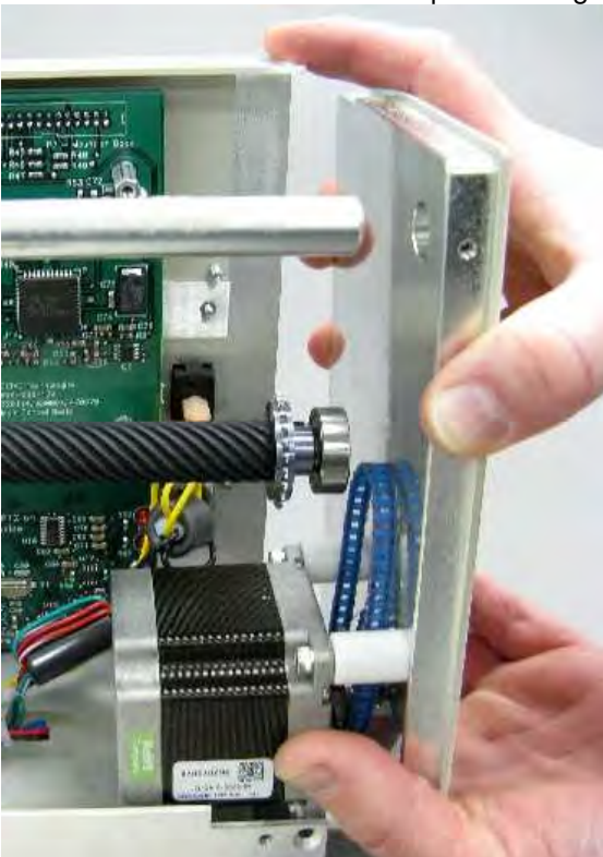
Figure 14. Removal of right end plate.
