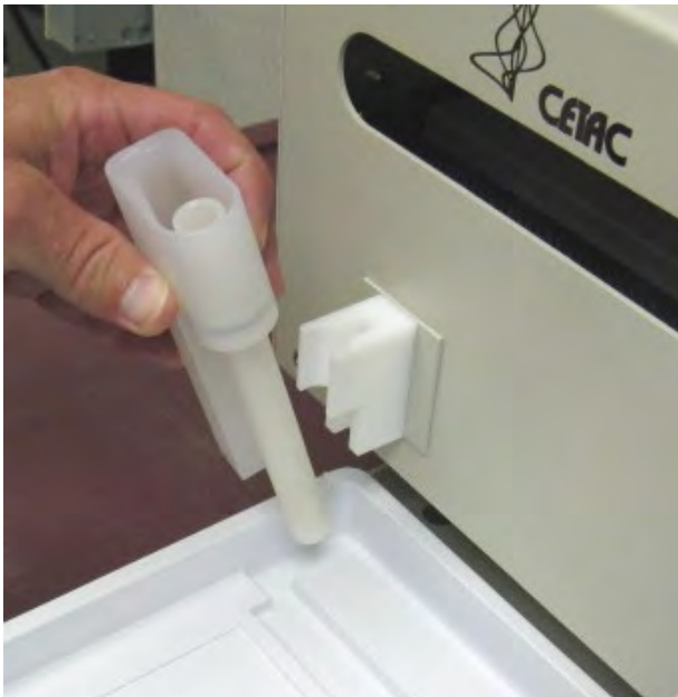
Figure 4. View of rinse station.
