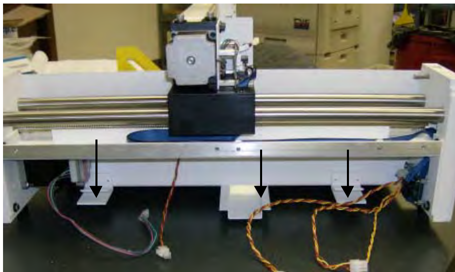
Figure 4-5. Cables disconnected and support brackets exposed.
