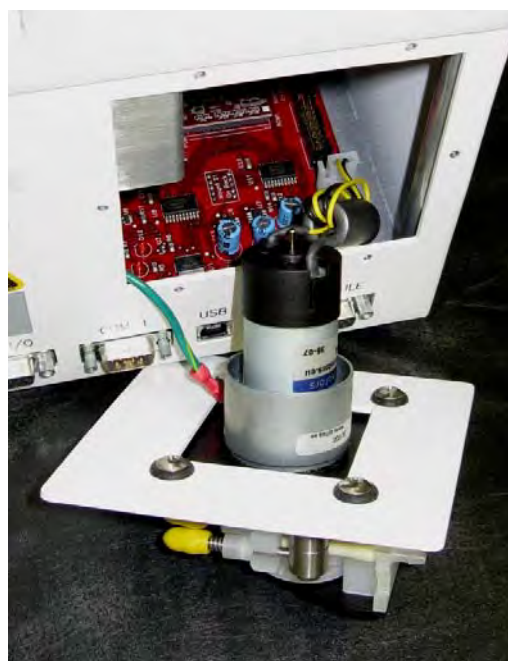
Figure 3-2. Pump mounting plate pulled away from chassis.
