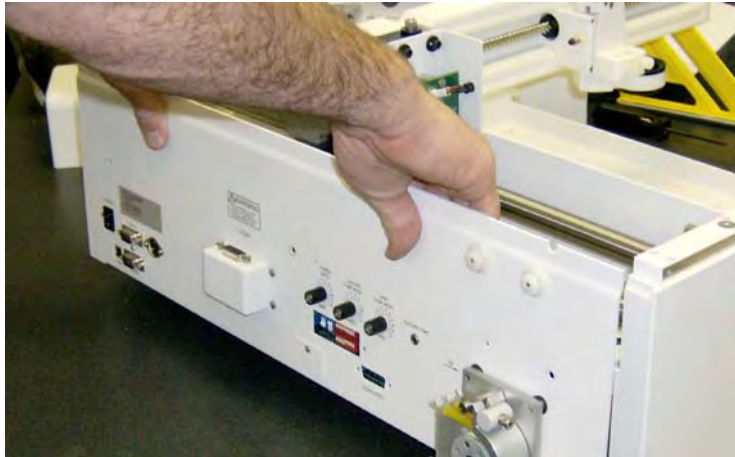
Figure 4-4. Removal of electronics panel.
