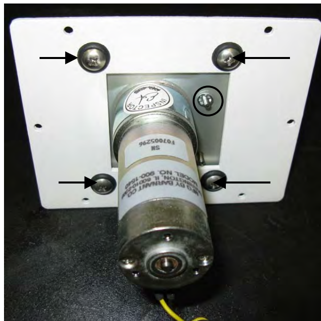
Figure 3-4. Older style pump in mounting plate. Note the grounding post for 3/8" nut.
