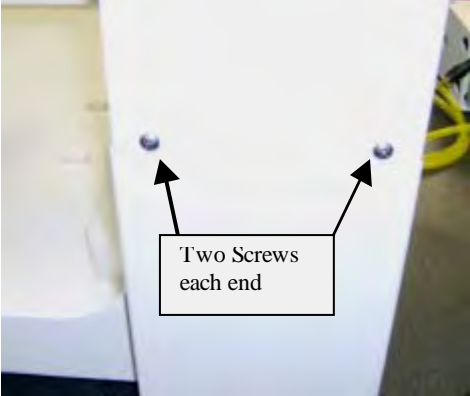
Figure 4-2. Cover mounting screws.
