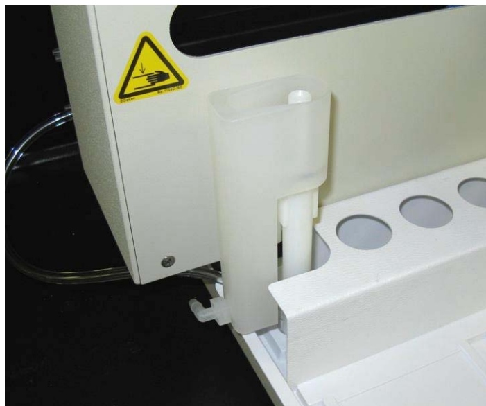
Figure 1-4. View of rinse station.
