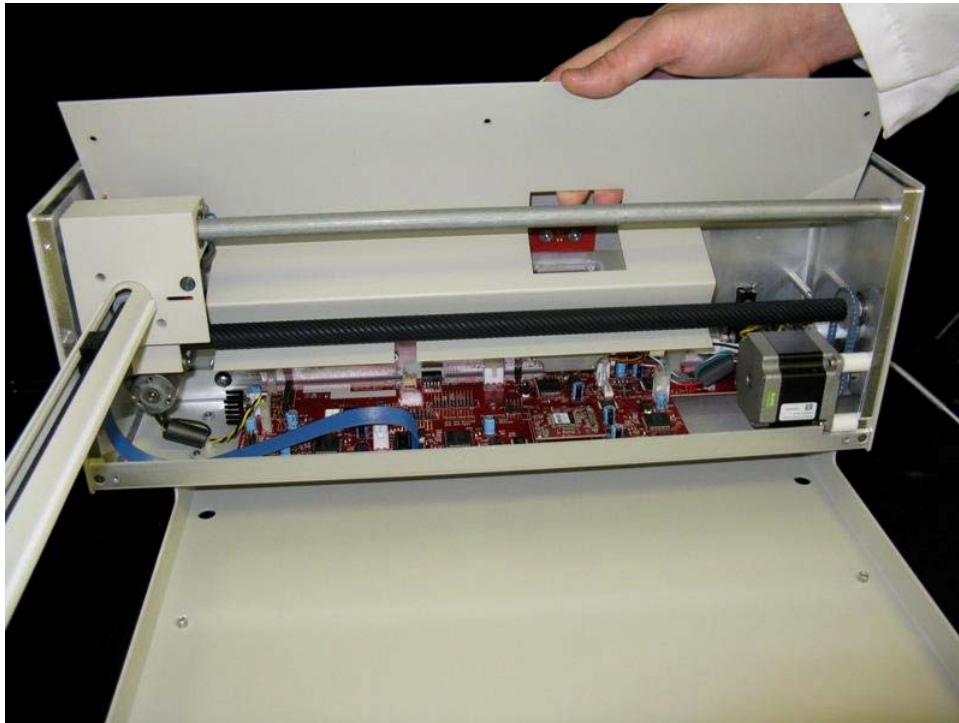
Figure 1-10. Removal of inner shield.
