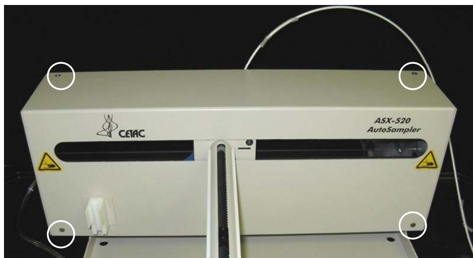
Figure 1-7. Front view of ASX-510 Auto Sampler showing front cover screws.
