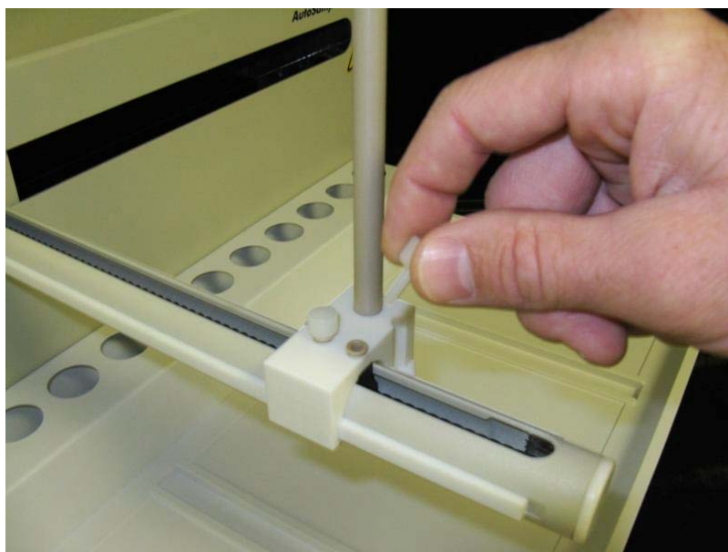
Figure 1-2. View of Y- axis home block with Kynar thumbscrews.
