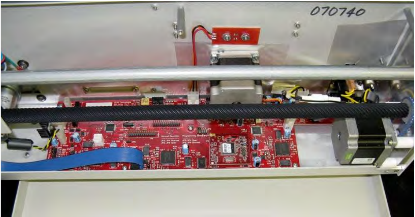
Figure 1-12. View of ASX-520 with inner shield removed.
