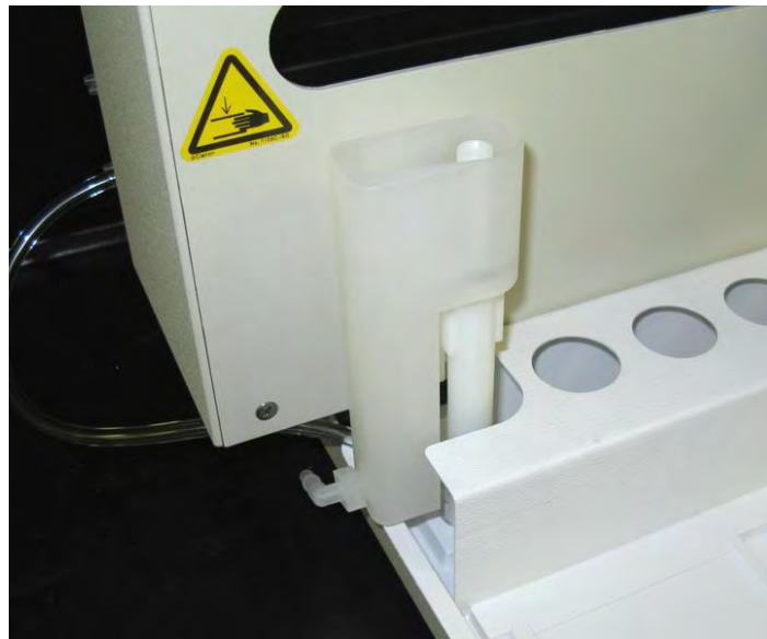
Figure 1-4. View of rinse station.
