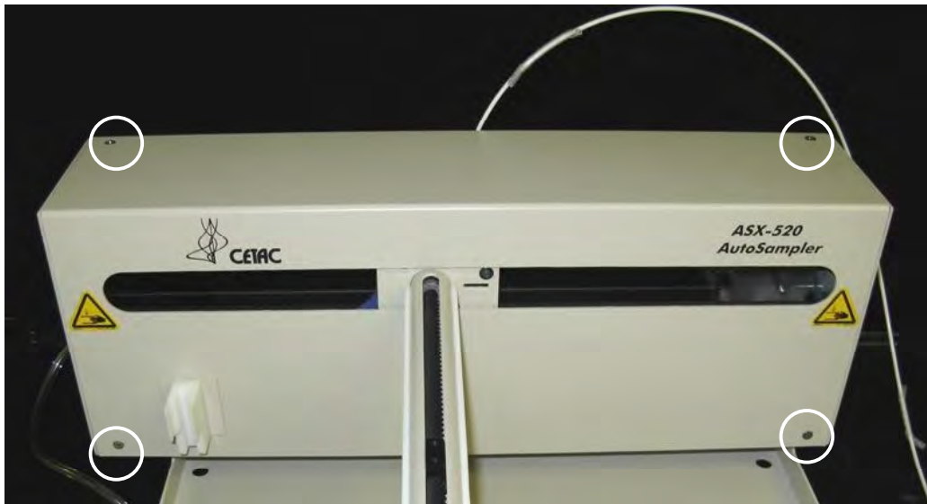
Figure 1-8. Front view of ASX-510 Auto Sampler showing front cover screws.
