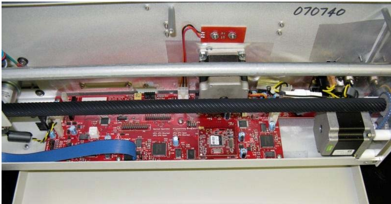
Figure 1-12. View of ASX-520 with inner shield removed (Rev 5 main board).
