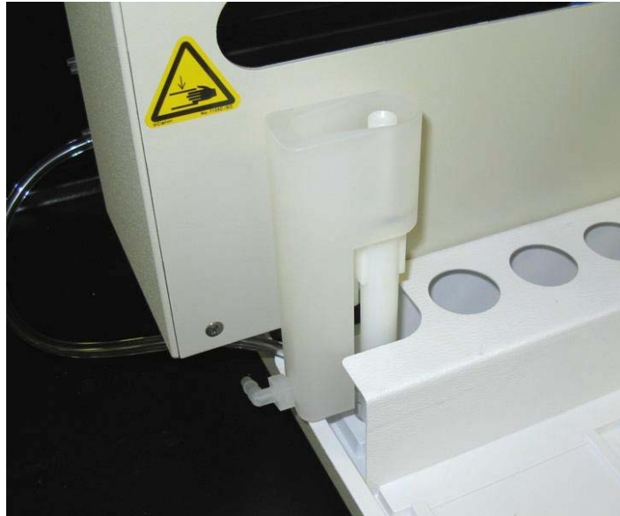
Figure 1-4. View of rinse station.
