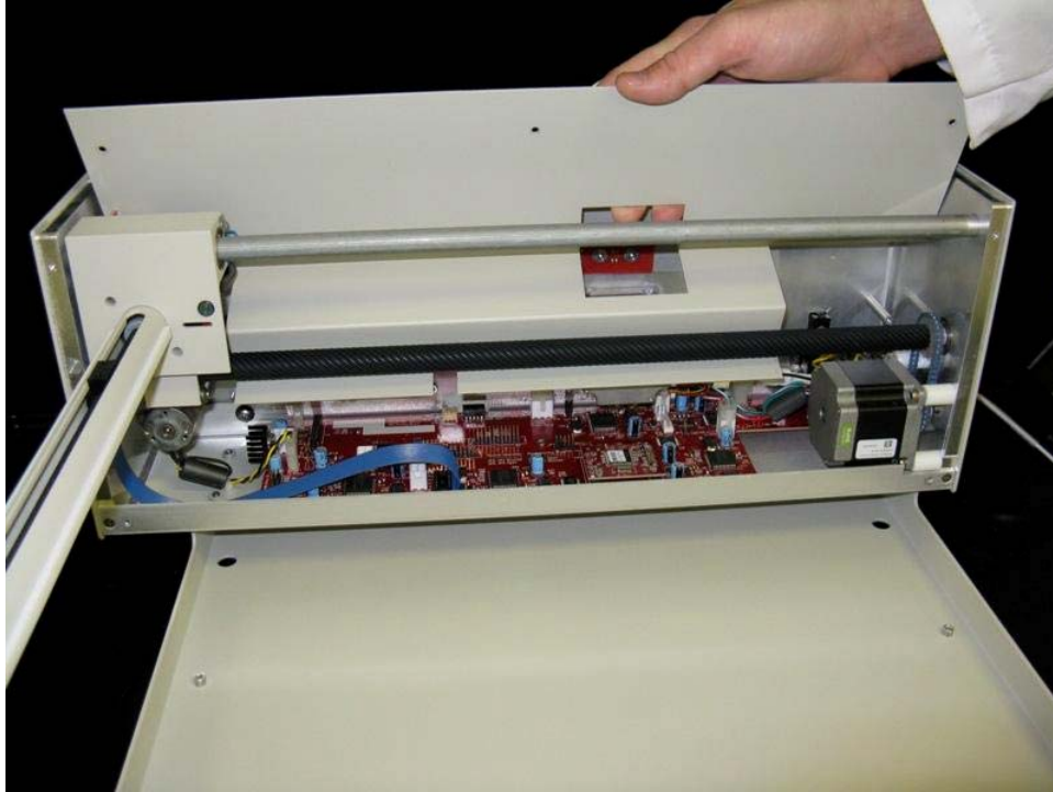
Figure 1-11. Removal of inner shield.
