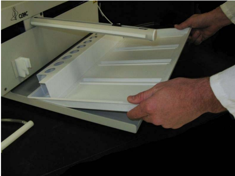
Figure 1-7. Removing the tray.
