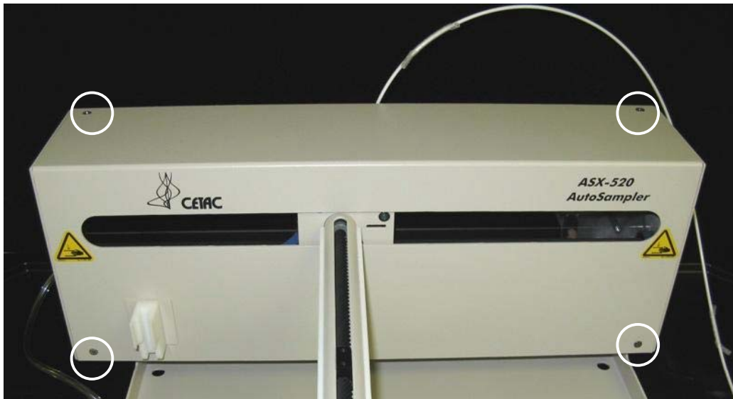
Figure 1-8. Front view of ASX-520 Auto Sampler showing front cover screws.
