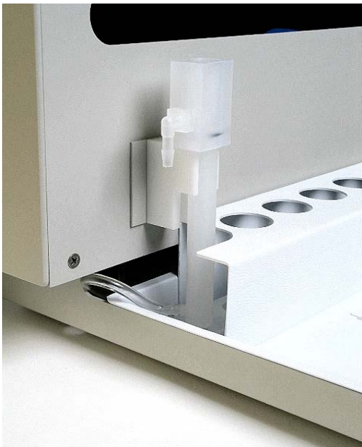
Figure 1-4. View of rinse station.
