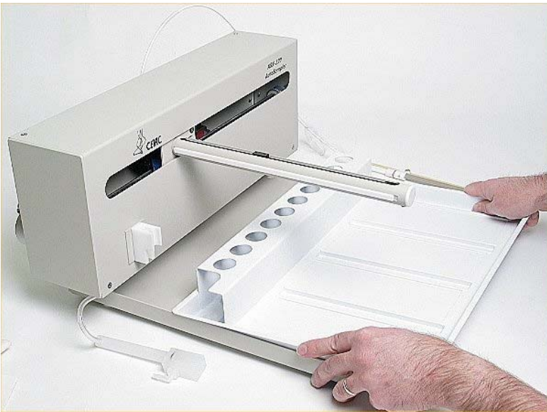
Figure 1-6. Removing the tray.
