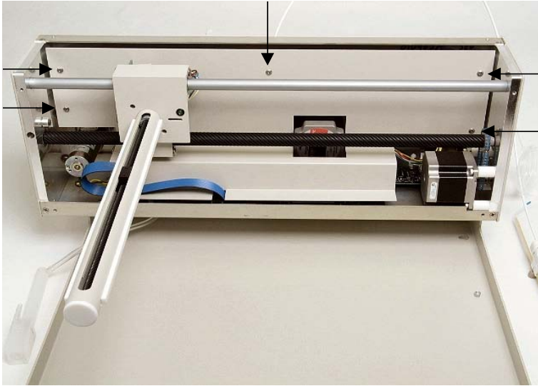
Figure 1-9. View of inner shield inside the ASX-520 Autosampler.
