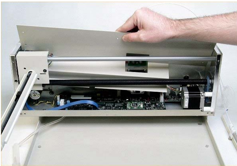
Figure 1-10. Removal of inner shield.
