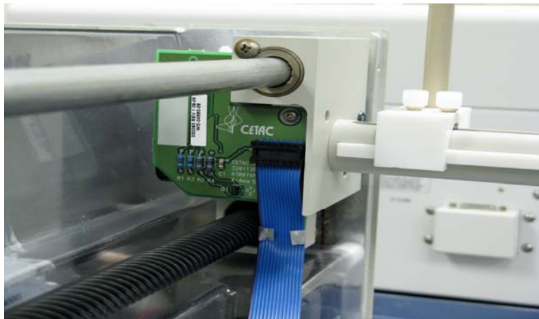
Figure 1-16. Ribbon cable connection to carriage assembly.
