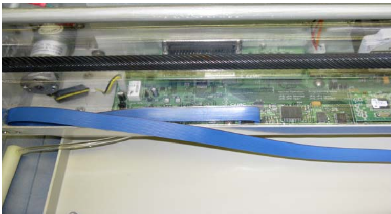
Figure 1-13. 31 inch ribbon cable installation.
