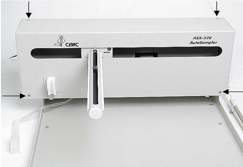
Figure 1-7. Front view of ASX-520 Autosampler showing front cover screws.
