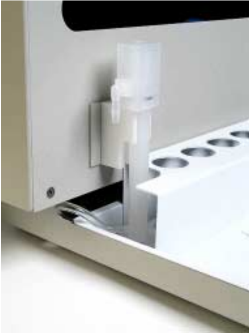
Figure 1-4. View of rinse station.
