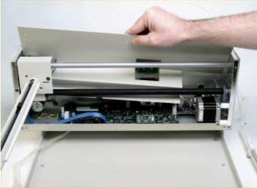
Figure 1-10. Removal of inner shield.
