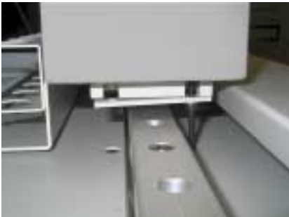
Figure 9. Attaching the right side of the head assembly.
