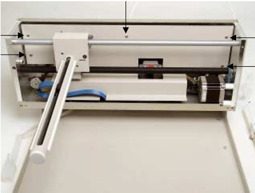
Figure 1-9. View of inner shield inside the ASX-520 Autosampler.
