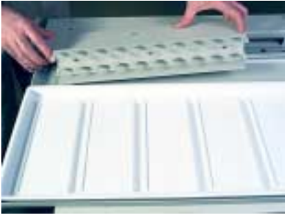
Figure 5. Standards rack placed onto the Extended Rack.
