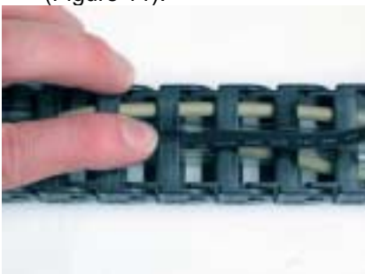
Figure 11. Inserting the power cord into the chain assembly.
