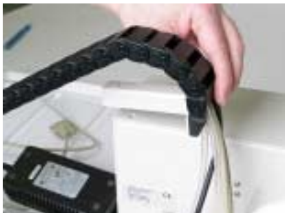
Figure 12. Attaching the chain assembly to the head assembly.
