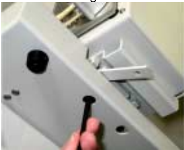
Figure 7. Attaching the head assembly (first screw).
