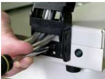
Figure 13. Attaching the chain assembly to the Extended Rack.
