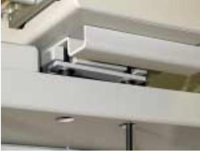
**Figure 8.** Attaching the head assembly (second screw).
