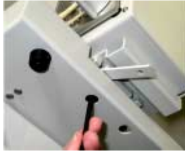
Figure 6. Attaching the head assembly (first screw).
