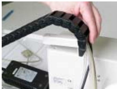
Figure 10. Attaching the chain assembly to the head assembly.
