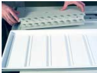
Figure 2. Standards rack placed onto the Extended Rack.
