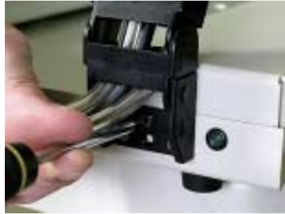
Figure 11. Attaching the chain assembly to the Extended Rack.
