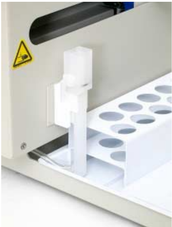
Figure 1-4. View of rinse station.
