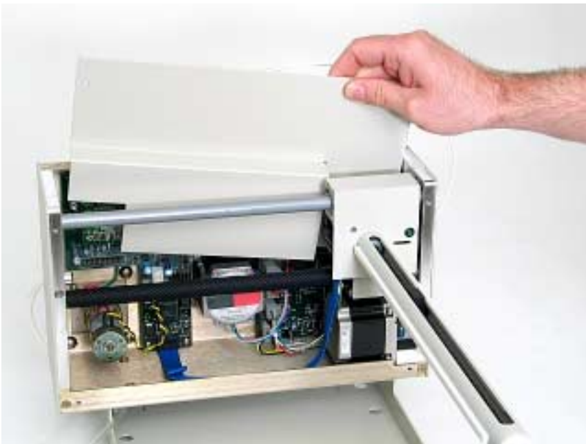
Figure 1-10. Removal of inner shield.
