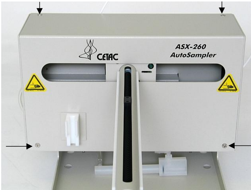
Figure 1-7. Front view of ASX-260 Autosampler showing front cover screws.
