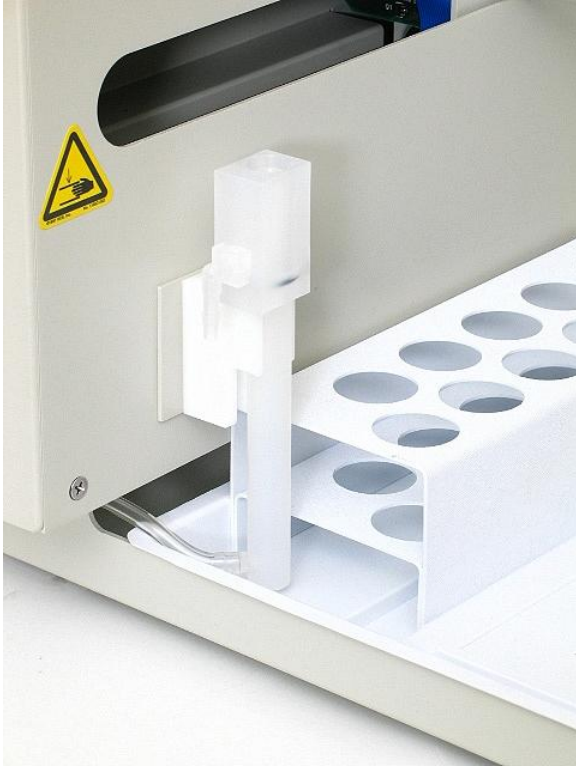
Figure 1-4. View of rinse station.
