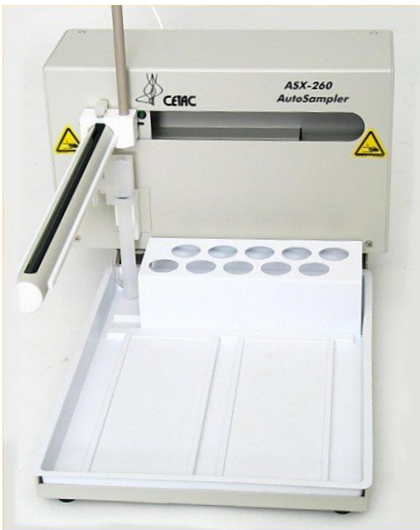
Figure 1-1. Front view of ASX-260 Autosampler.
