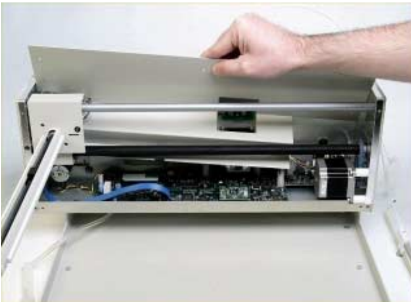
Figure 1-10. Removal of inner shield.
