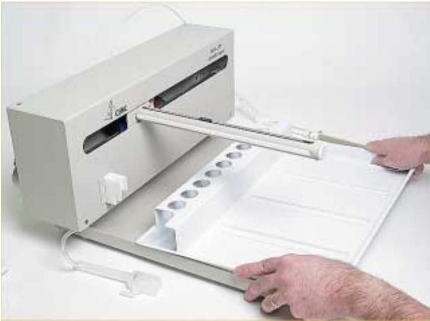
Figure 1-6. Removing the tray.
