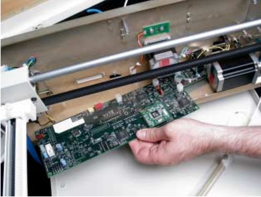
Figure 1-18. Removal of main board.
