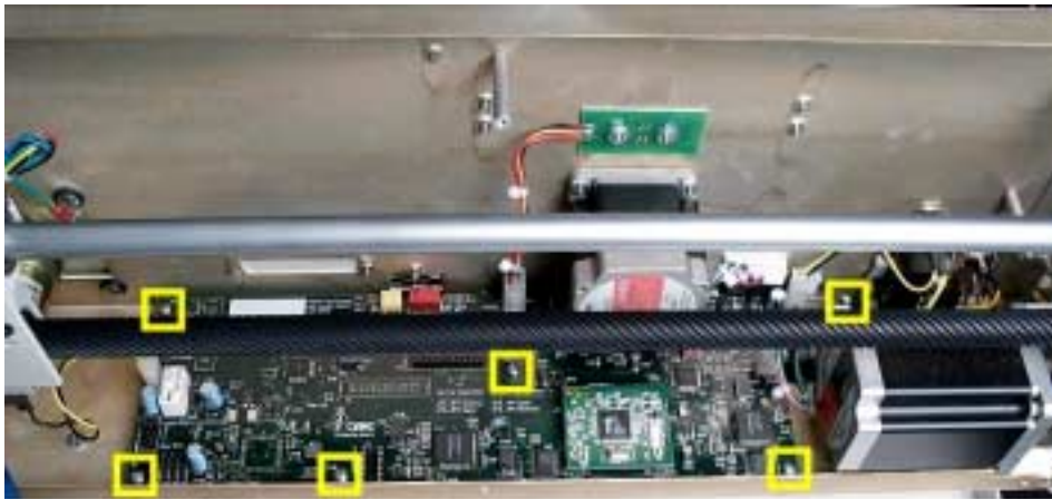
Figure 1-14. Main board with screw locations.
