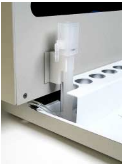
Figure 1-4. View of rinse station.
