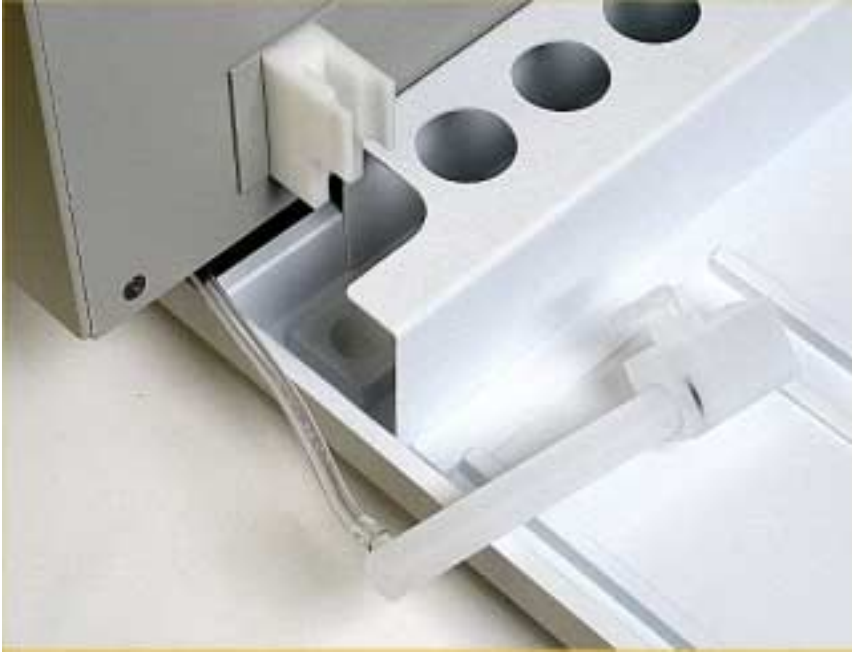
Figure 1-5. View of rinse station removed from the front cover.
