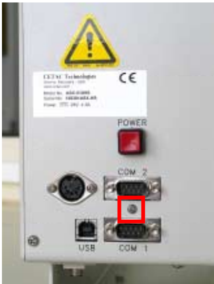
Figure 1-15. Screw below COM 2 port.
