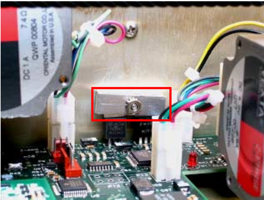
Figure 1-17. Heat sink bracket.
