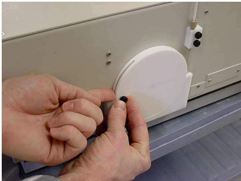
Figure 6. Securing peek tubing to rotor.
