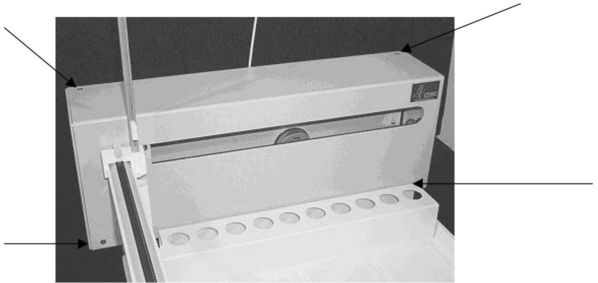
Figure 1-7. Front view of ASX-510 Auto Sampler showing front cover screws.
