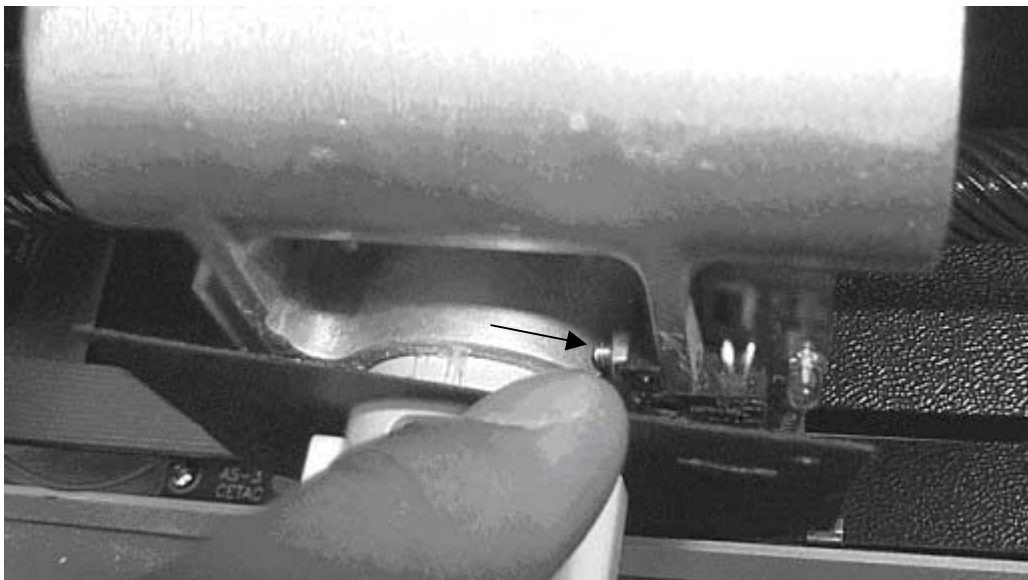
Figure 1-14. Top view of Y-axis sensor showing mounting nut and screw.
