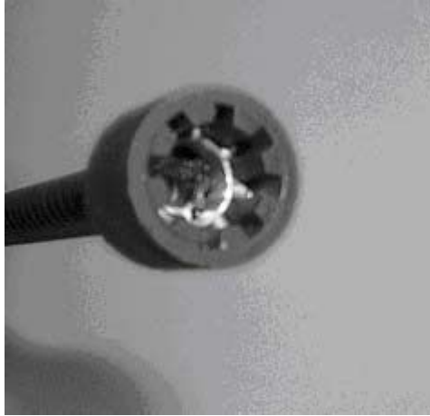
Figure 1-11. Keyed end of flex coupling on the Y-Axis leadscrew.
