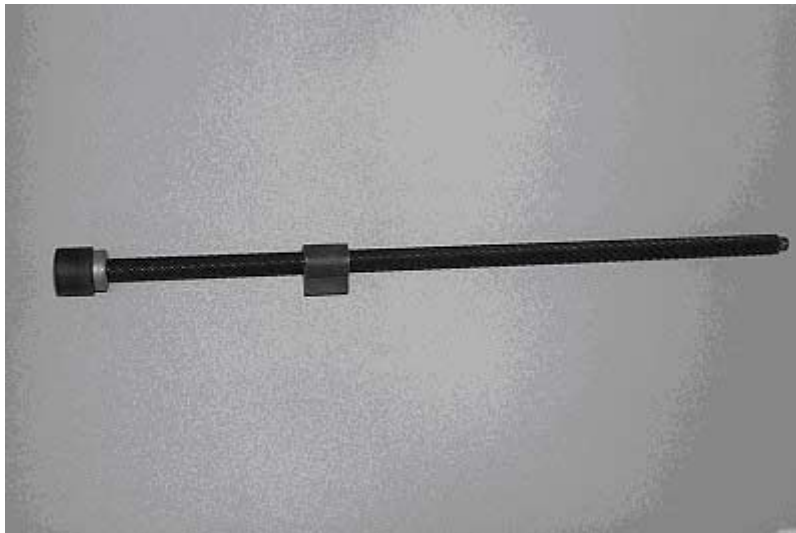
Figure 1-10. Y-Axis leadscrew with nut and flex coupling attached.
