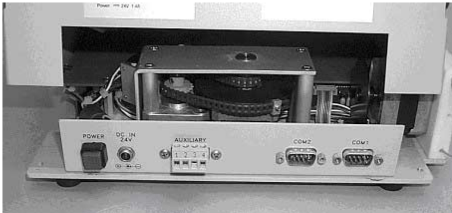
Figure 1-10. Back view ASX-100 showing I/O panel.
