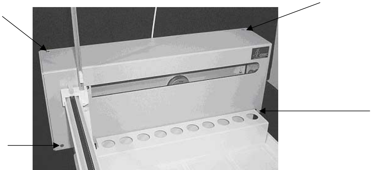
Figure 1-7. Front view of ASX-510 Auto Sampler showing front cover screws.
