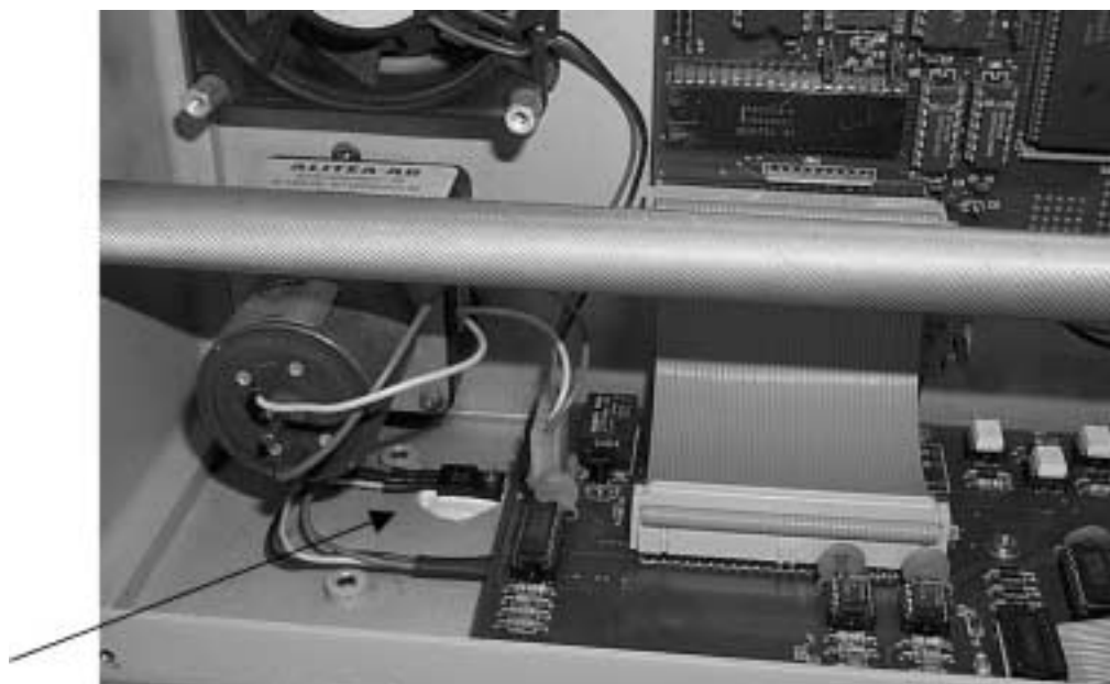
Figure 1-12. View of ASX-510 showing old style pump.
