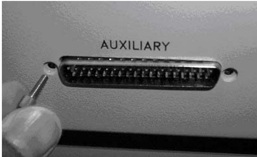
Figure 1-17. Back view of connector that attaches to the Daughter board.
