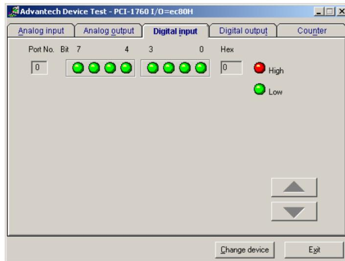
On the laser system, use a Single Point pattern at 5% energy with a Burst Count of 1. Draw a few spots on the sample (e.g. 10), and open the sequence editor. Set the trigger delay to zero seconds and run the sequence. The indicator under '0' in the Advantech Device Test window should turn red whenever the trigger is sent from the laser. NB: This corresponds to Input ID 1 in PlasmaLab.
