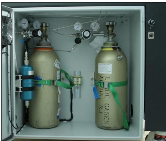
The ATLEX short pulse excimer laser used in the Analyte G2 requires two dedicated gas bottles for operation: ArF laser gas and He flush gas. These bottles remain permanently attached to the laser. Provisioning for the correct gas bottles is an essential part of site preparation.
