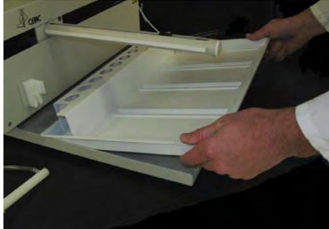
**Figure 2-6.** Removing tray from autosampler
