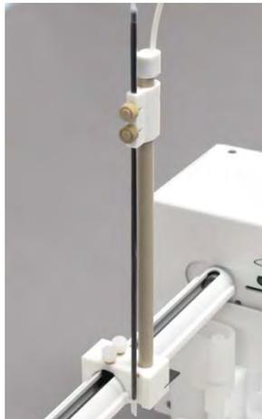
**Figure 3-2.** Z-Drive Assembly with Z-Axis Slider.
