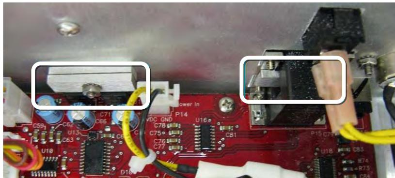
Figure 2-13. Heat sink nut and comm. port retaining strap
