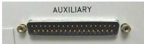
**Figure 2-1.** Auxiliary I/O Card with Male Connector
