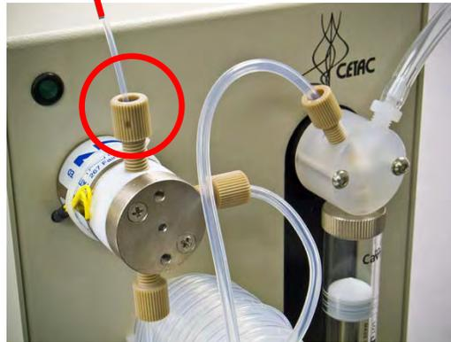
**Figure 3-5.** Autosampler Probe Connection to Solenoid Valve.
