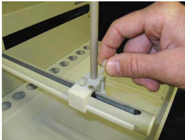
**Figure 2-3.** View of Y-axis home block with Kynar thumbscrews
