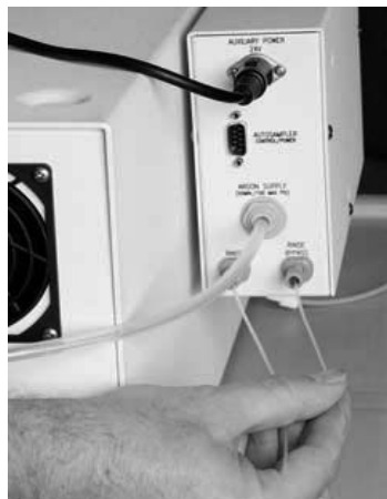
Figure 3d. Connections to QuickWash Accessory – Manual Operation.
