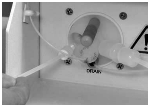
Figure 4c. Connection of Gas/Liquid Line to Spray Chamber.
