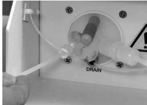
Figure 3c. Connection of Gas/Liquid Line to Spray Chamber.
