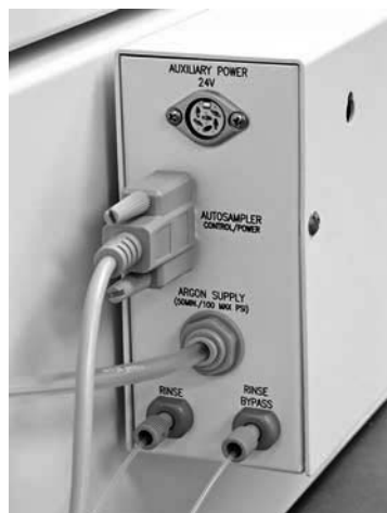
Figure 4d. Connections to Back of QuickWash Accessory.
