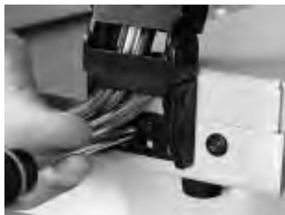
**Figure 3-11.** Attaching the chain assembly to the Extended Rack.
