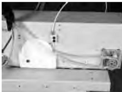
**Figure 3-12.** Connecting the pump tubing.
