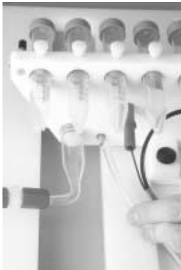
Connection of waste line to bottom of flush port.
