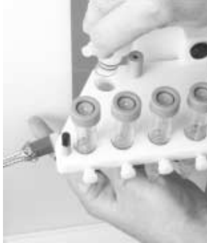
Insertion of nebulizer into spray chamber.
