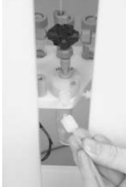
Nebulizer gas line connection.
