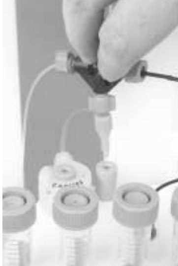
Connection of crosspiece to flush port.
