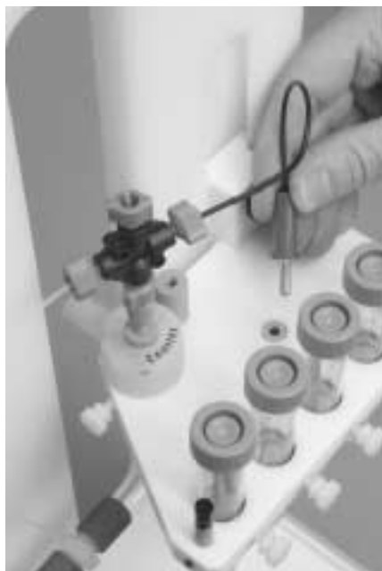
Top view, ground cable connection.
