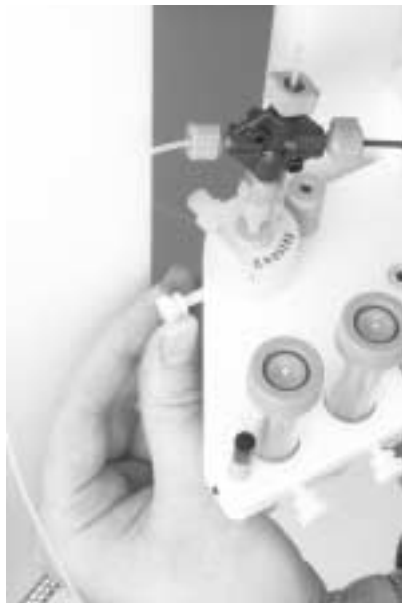
Thumbscrew to secure nebulizer.
