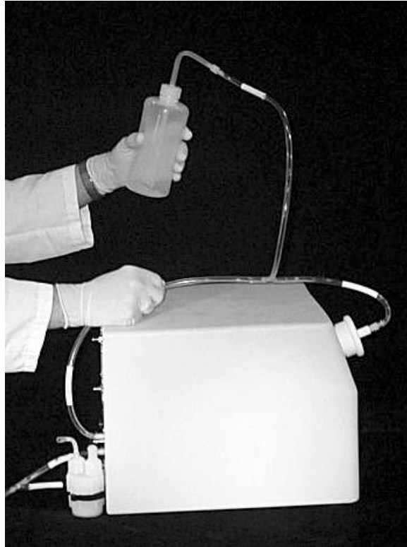
Figure 6-1. Membrane system rinse diagram.
