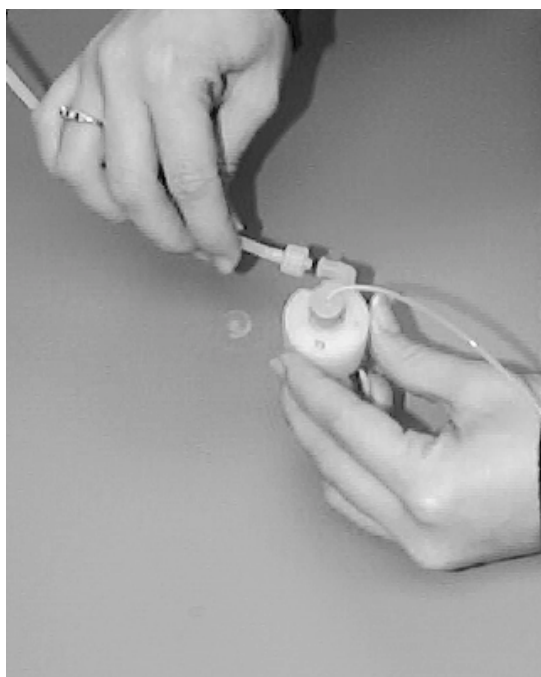
Figure 3-4. Connecting the nebulizer gas line.
