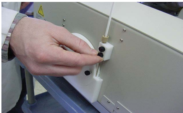
Figure 5-2. Securing block to back of autosampler.
