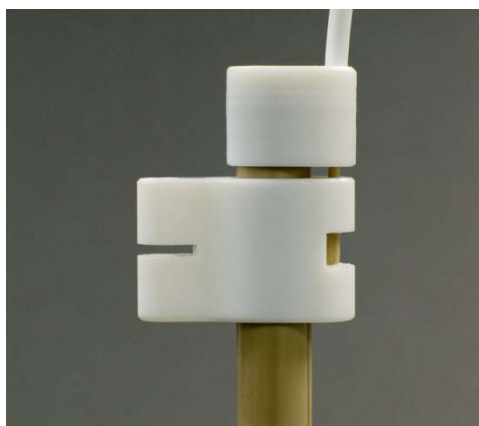
Figure 5-3. View of gap between probe bracket and cap (standard Z-drive).
