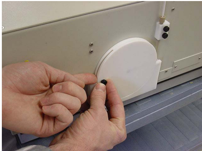
Figure 5-4. Securing cable to rotor (PEEK cable).
