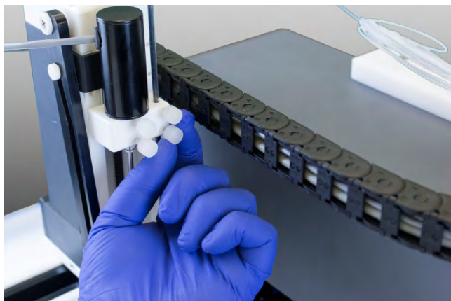
FIGURE 9 Installing the Probe
