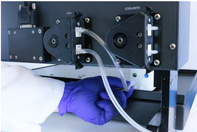
FIGURE 13 Connecting the Rinse Station Drain (Oils Side Is Shown)
