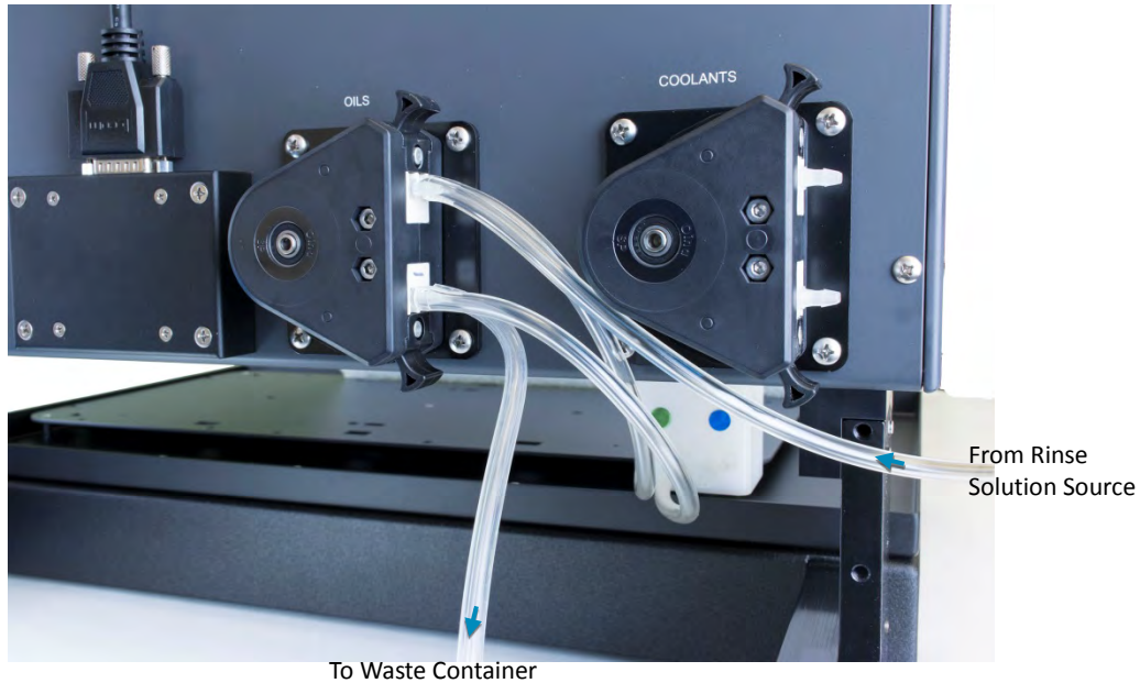
FIGURE 15 Completed Rinse Station Tubing for the Oils Side
