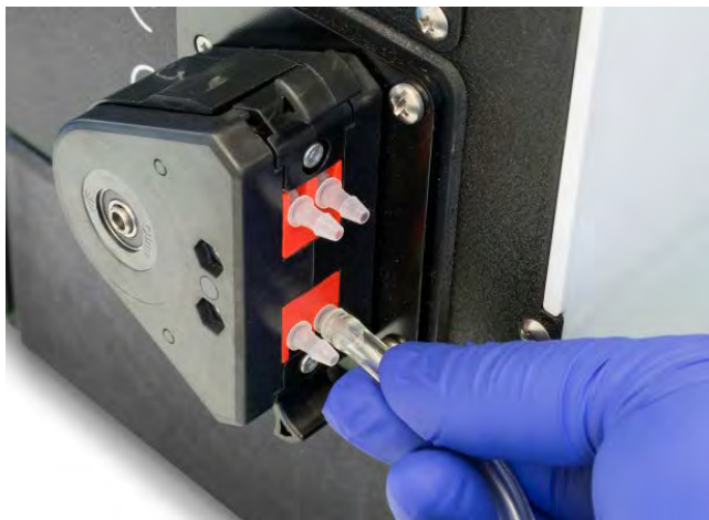
FIGURE 11 Connecting the Waste Line
